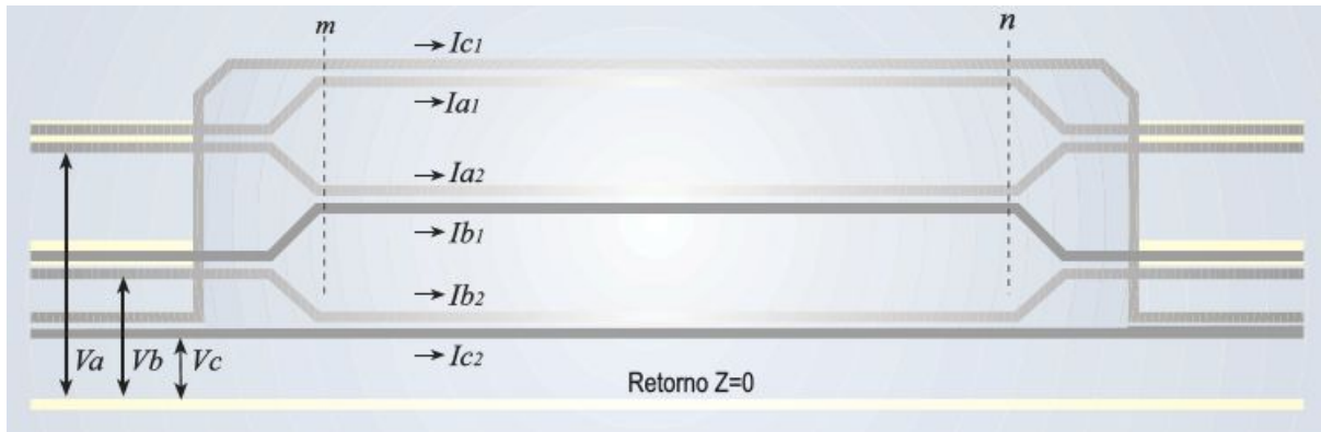
Figure 4. Every current is divided into two sub-currents. Then, the paired-phase system is accomplished.
